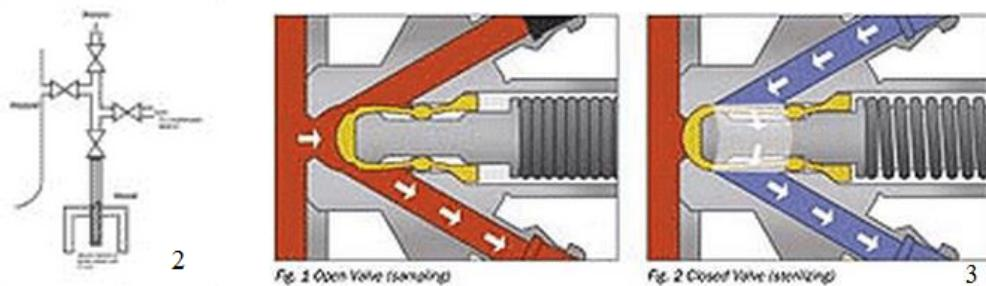
In principle, variant 2 can be realized by the laboratory staff. Variant 3 is a compact, and seems to be elegant and a simple solution, but for its realization high accuracy and professionalism is required. A wide range of industrial sampling valves operates according to this principle.
