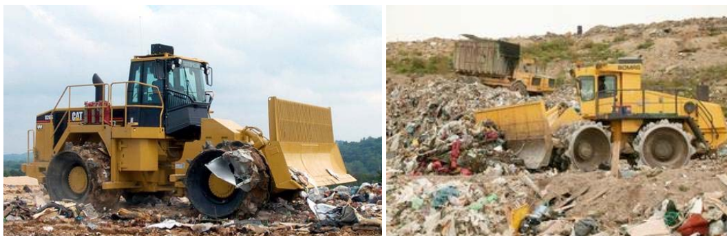
Figure 6.2-2 Various types of landfill compactors 2
