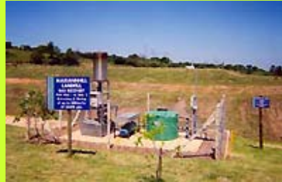
Mariannhill landfill gas recovery and flaring station (Photo: World Bank)
